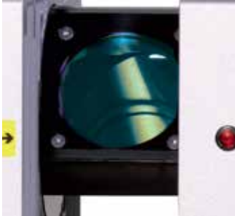
Rotating mirror for 310° vertical scanning
